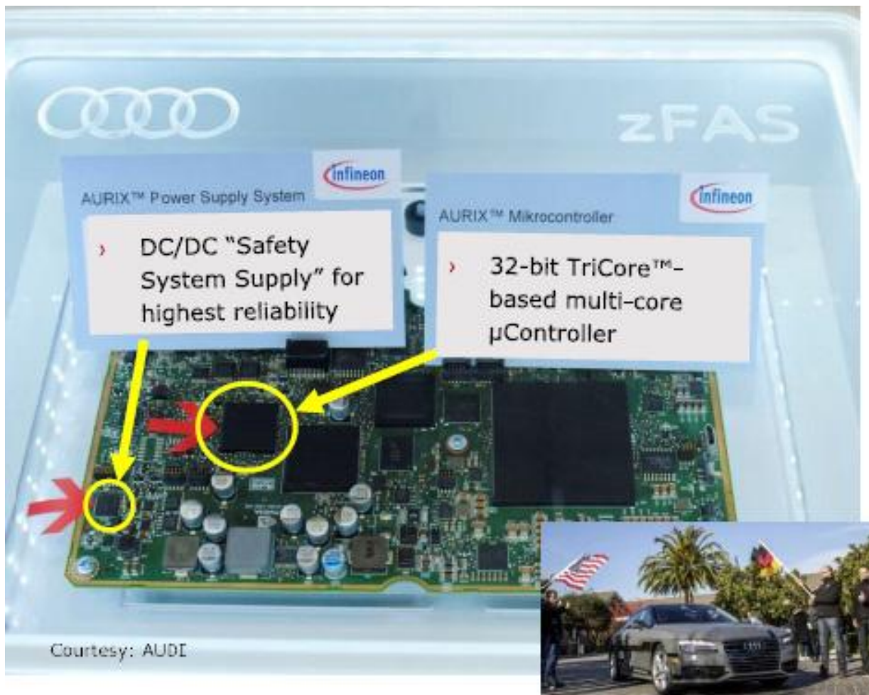
Figure 34: Sensor fusion box an opportunity for GPU, microcontrollers, power semis
