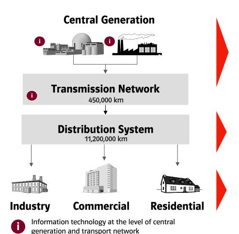
Supply and demand balancing takes place between central generation and transport grid Generation output following demand
