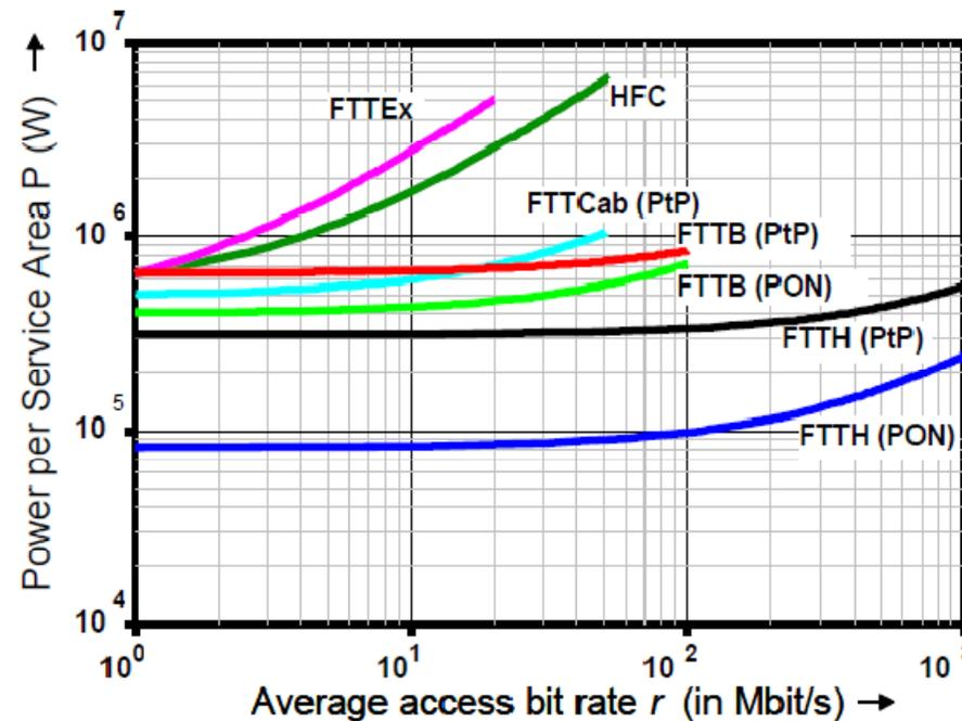
Figure 2: Power  $P$  per dense urban service area as a function of the average access bit rate  $r$
