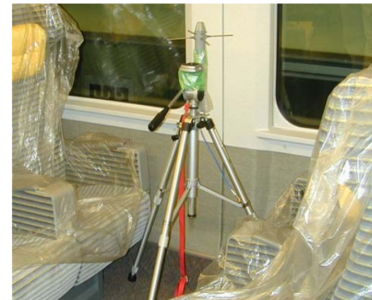
Receiving Antenna (Cross dipole, Omni-directional)
