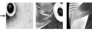
81 images in total, 156 scratch defects, 64 images (120 defects) for and 17 images (36 defects) for verification
