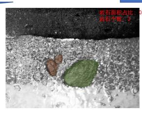
Use Unet Network for image segmentation on the pixel level. Divide the image as rock areas and background areas. Then, calculate the size and number of rocks.
